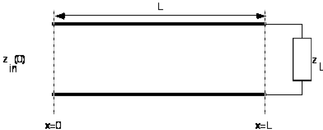
Figure 4. Input impedance of a loaded transmission line.
